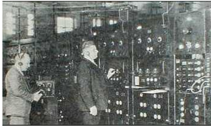
Figure 2.1. H.O. Peterson and H. H. Beverage and their triple diversity HF receiver (1933)
