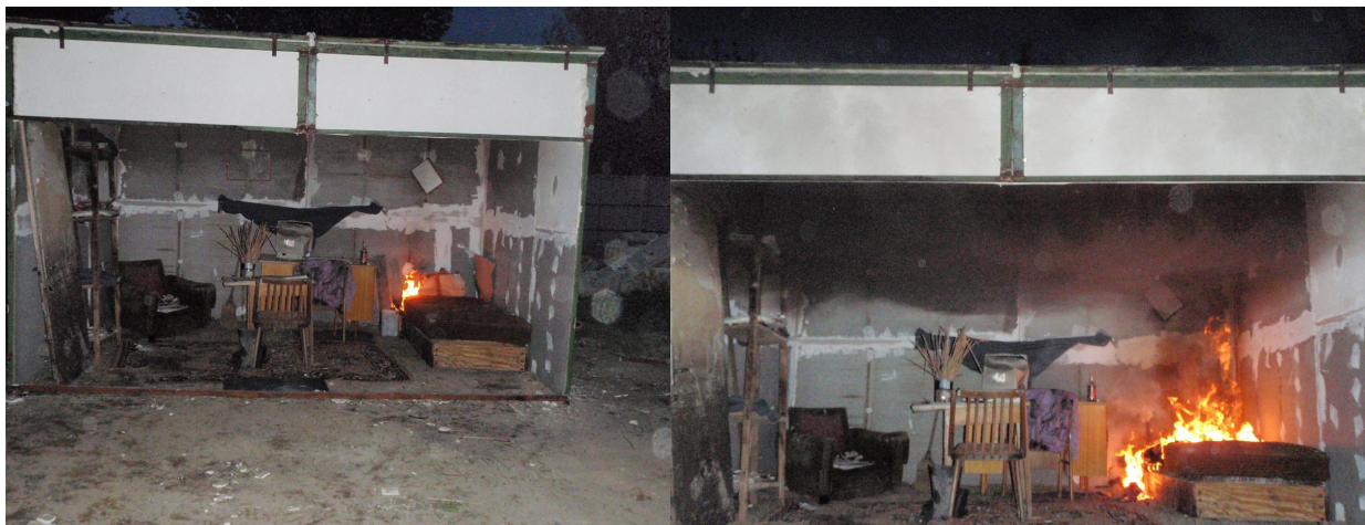
Pictures 8-9. Light-structure fire drilling facility with initial fire and forming of “fire-blanket” at the Berettyóújfalu Fire Department, Own picture
