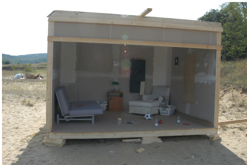
Picture 7. “Fire-cell” built for examining closed area fire (Source: Fire Department, Pécs, Hungary, 2009.)
