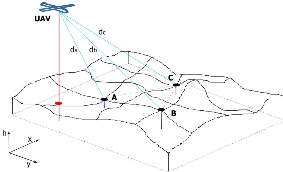
Figure 6. Coordinates of the UAV and the known base points of the terrain
