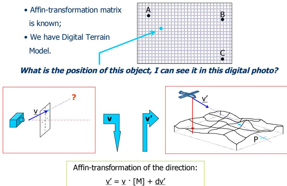
Figure 8. Calculating of the stab point on the fundamental level
