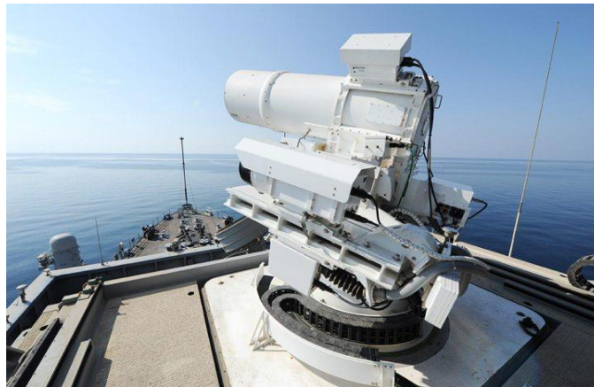
Figure 4: LaWS – Laser Weapon System integrated into US Marine’s existing ship defence systems in September 2014.(Photo: DMN) 27 [18]
