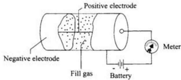
Fig. 2. Basic elements of gas-filled detector (from Valković)
