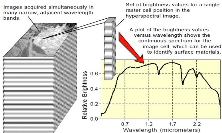
**Fig. 4.** General principle of hyperspectral imaging - ©MicroImages, Inc., 1999-2012
