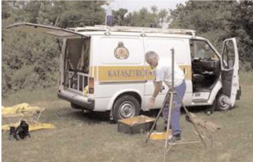
Figure 6. Special car of disaster recovery for deploying and collecting data of chemical probes
