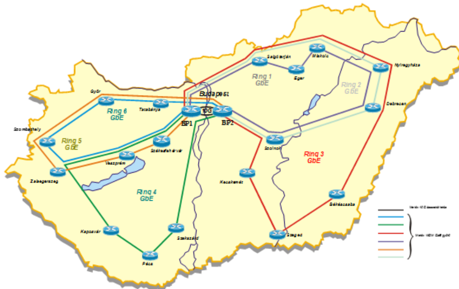
Figure 2. The DWDM (Dense Wave Division Multiplexing) high speed optical ring communication topology in Hungary, in common with emergency networks
