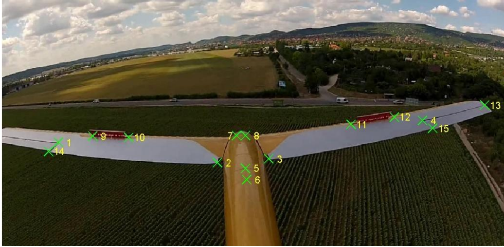
Figure 4. Visual reference points used for Head Up Display boresighting
